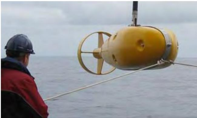
*Figure 4. The SOCRATES towed sonar source being deployed.*
