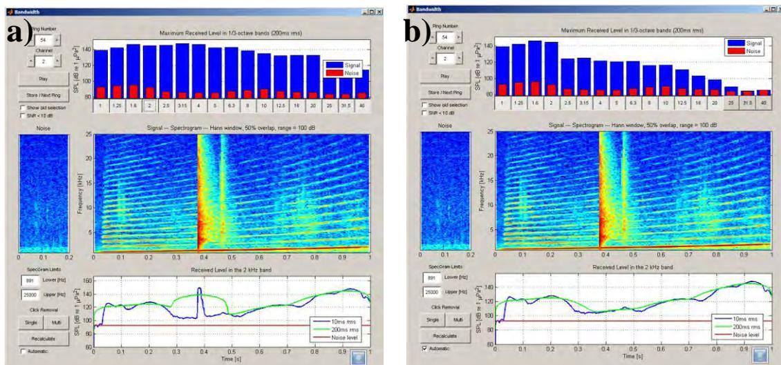
**Figure 8.** The automatic selection of 1/3-octave bands using the 10 dB SNR criterion a) before, and b) after removal of a sperm whale click. The blue and red bars in the upper panel show the  $SPL_{max}$  of the signal and SPL of the noise segment, respectively, for bands with centre frequencies of 1 to 40 kHz. The toggle buttons below the bars indicate if a band passed the SNR criterion and was selected for the calculation of the sound levels.
