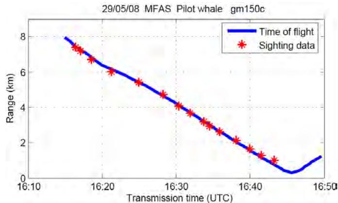
**Figure 10.** The „time-of-flight“ range function is fitted to the „sightings“ range data to determine the distance from source to whale over the entire exposure run.
